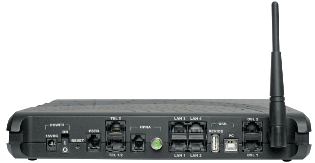
Scientific Atlanta's DDR2000 xDSL Residential Gateway Back Panel
